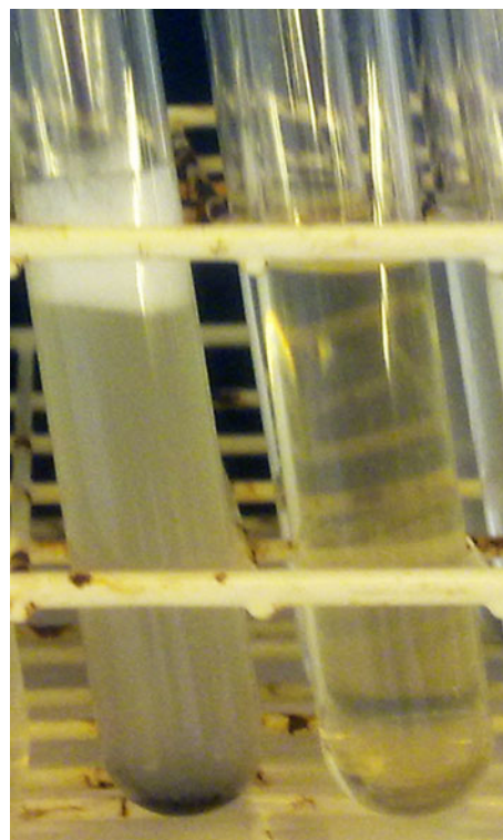
Fig. 5 Anaerobic culture tubes with an initial glycerol concentration of 98 g/l stored crude glycerol (batch I) after 20 h of incubation. Activated stone carbon was included in the left tube
